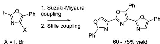
A regioselective Suzuki–Miyaura cross-coupling of 2,4-dihalooxazoles followed by a Stille coupling has been successfully developed. The procedure affords convergent syntheses of trisoxazoles in high yield and in a minimum number of steps.
